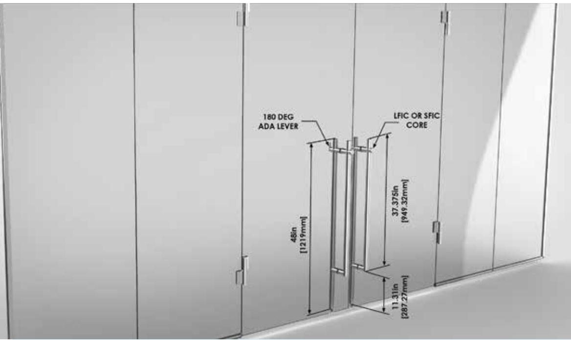
This schematic shows a 180-degree ADA staggered level handle pull. The lever pull handle rotates only 180 degrees without push-button actuation and must be easy to turn with one hand without the need for tight grasping, pinching or turning of the wrist. It must be designed and installed no more than 1220 mm (48 inches) above the finished floor with a minimum height of 965 mm (38 inches).
